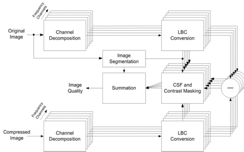
**Fig. 1.** Block diagram of the HVS model
