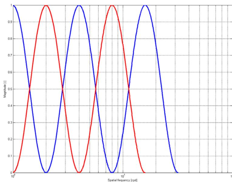
**Fig.2.** Filter bank of 1-octave-wide cosine log filters . Note also the symmetry of the cosine log filters on a logarithmic scale.
