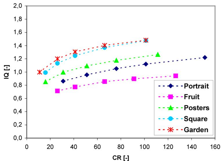
**Fig. 4.** The output of the model for five JPEG2000 compressed images at different compression ratios. Higher IQ values correspond with higher image distortions. IQ=0 is for original image.
